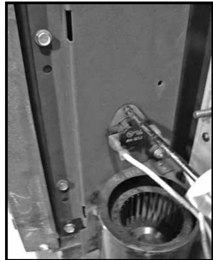
Figure 22: Unscrew thermal snap switch.
